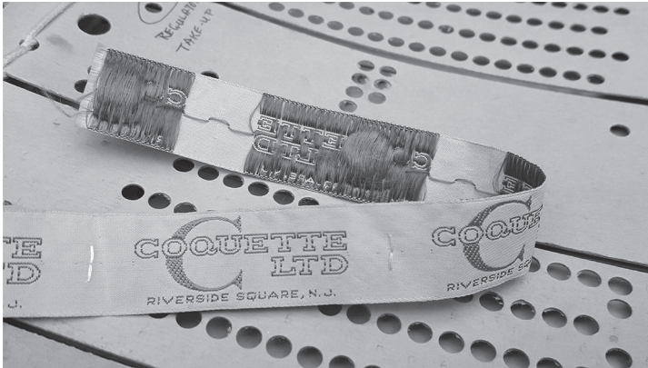
2.1a and 2.1b Stack of Jacquard cards used to produce the “Coquette” label and the finished label, n.d.
