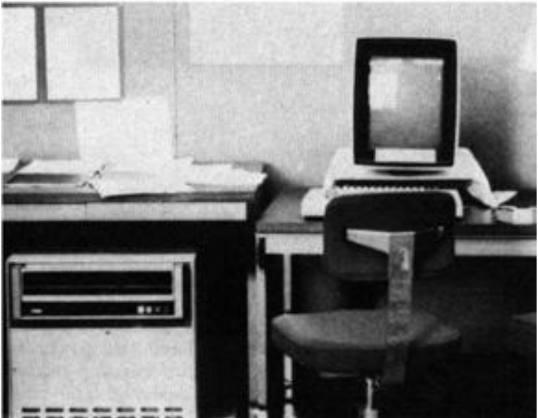
“The interim Dynabook system consists of processor, disk drive, display, keyboard, and pointing devices.” (The original caption from the article.)
